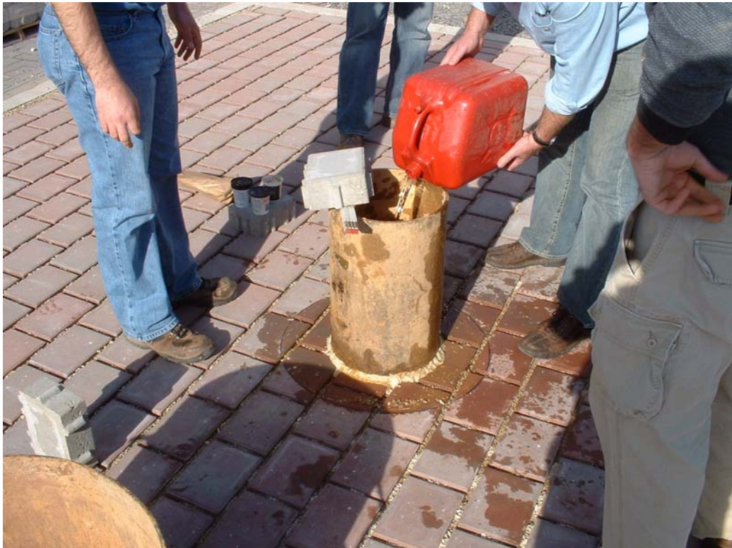
Surface inundation test
