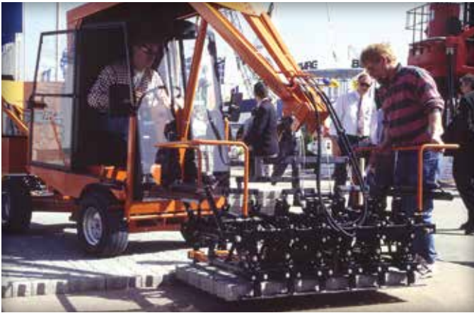
Figure 3. Motorized equipment with a mechanical clamp.
