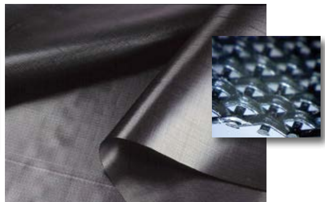
Figure 12. Woven mono-filament geotextile with close-up
