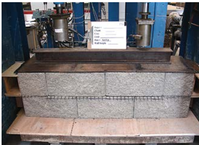
Figure 19. Geogrid connection testing with SRW units
