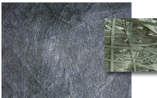
Figure 15. Non-woven heat bonded geotextile with close-up
