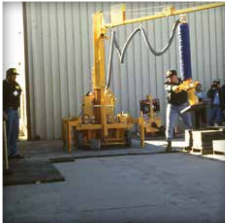
Figure 20. Vacuum assisted mechanical equipment for installing paving slabs.
