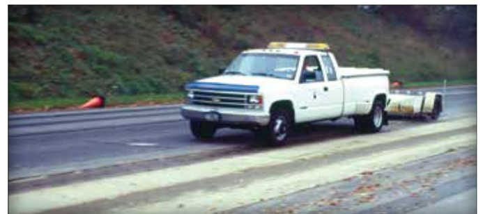
Figure 4. ASTM E 274 Test Equipment consists of a truck and trailer assembly. A tire within the trailer is towed at a given speed, locked, and skidded across water dispensed on the pavement in front of it.
